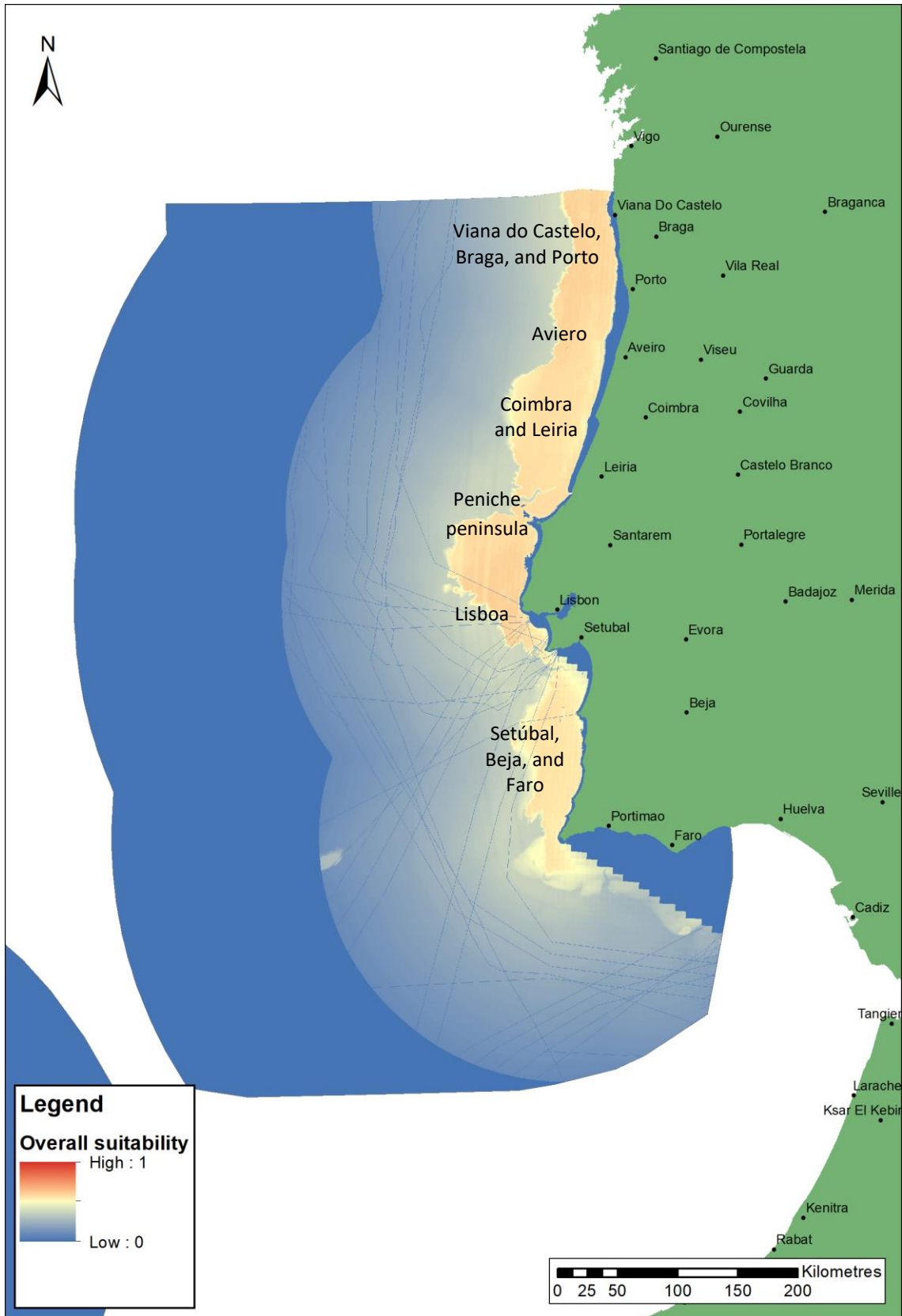
Figure 8. Overall suitability map for Portugal wave energy, with regions of highest resource labelled.
